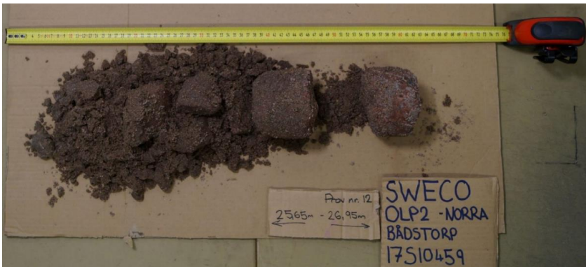
Figure 18. Borehole 2: Samples from Geobor-S triple tube sampling at a depth of 25.65 – 26.95 m (modified after Trafikverket, 2018).
