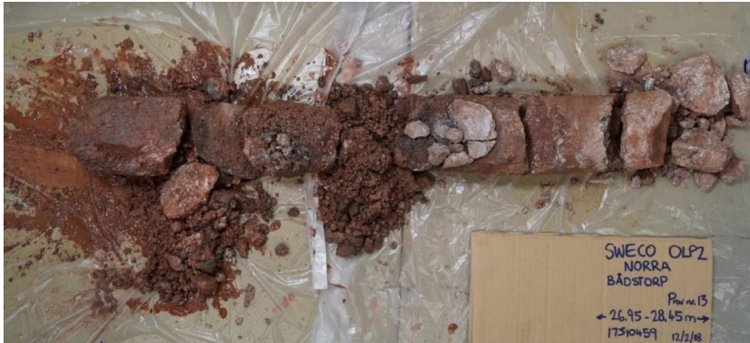
Figure 19. Borehole 2: Samples from Geobor-S triple tube sampling at a depth of 26.95 – 28.45 m (modified after Trafikverket, 2018).
