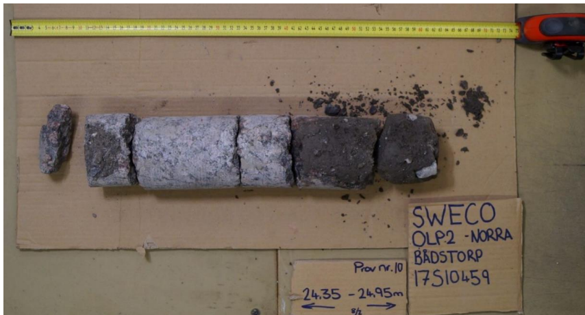
Figure 16. Borehole 2: Samples from Geobor-S triple tube sampling at a depth of 24.35 – 24.95 m (modified after Trafikverket, 2018).
