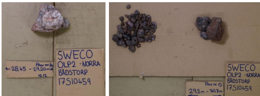
Figure 20. Borehole 2: Samples from Geobor-S triple tube sampling at a depth of 28.45-30.70 m (modified after Trafikverket, 2018).
