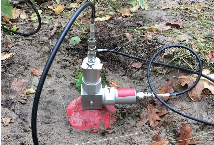
Figure 3. Vertical and horizontal vibration sensors mounted on a steel plate.
