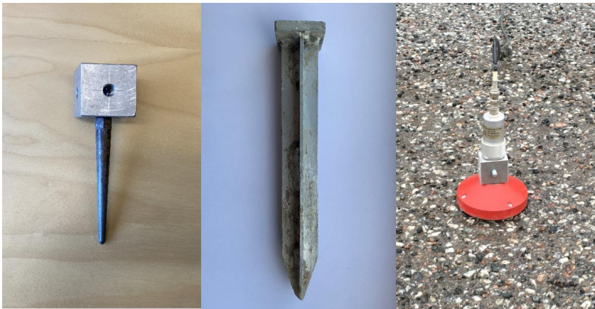
Figure 11. The three different mounting techniques. Soil pin (left), metal stake (middle) and steel plate (right).
